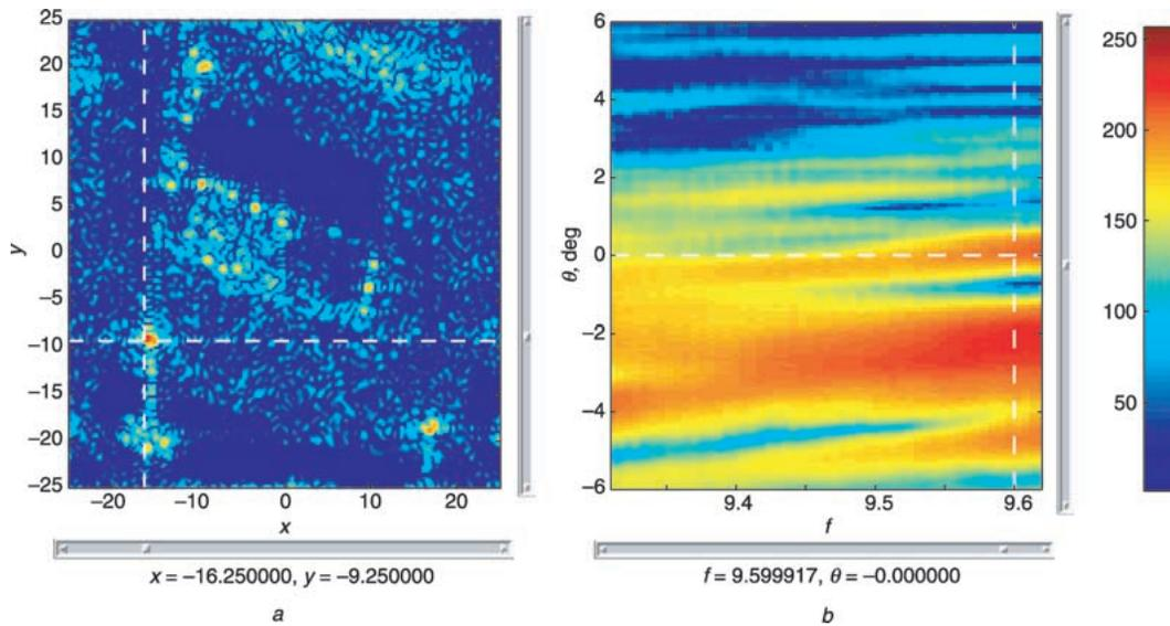
**Fig. 9** Frequency and angular behaviour of a bottom of a pylon located at ( $x = -16.25$  m,  $y = -9.25$  m)
