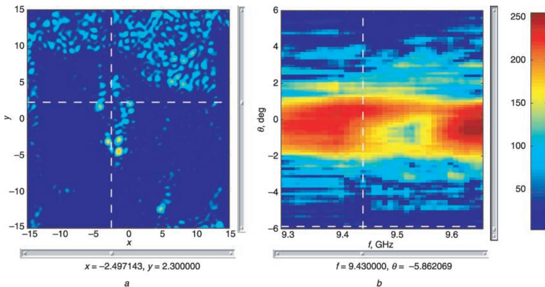
**Fig. 4** Variation of spatial SAR image for a given angle  $\theta = -5.86^\circ$  and frequency  $f = 9.43$  GHz
