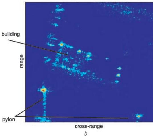
**Fig. 3** SAR images of aircraft type target (a) and building with some pylons around (b) built by the RMA algorithm
