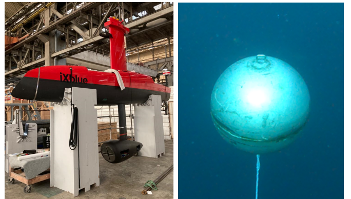
Fig. 2. Exail’s DriX USV (left): The cross-shaped linear arrays are visible in the gondola. The real target in open water (right): a metallic sphere of target strength TS = -15 dB.
