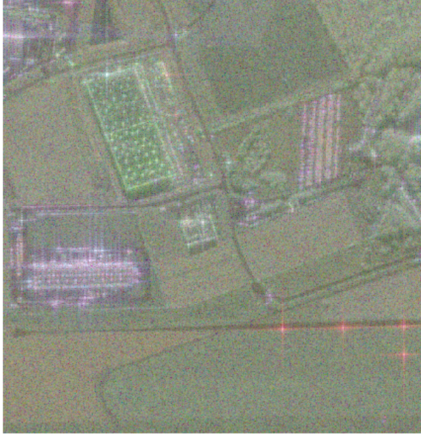
Fig. 1. Color representation of the Brétigny area, France in the Pauli basis : HH - VV in red, HV in green and HH + VV in blue.
