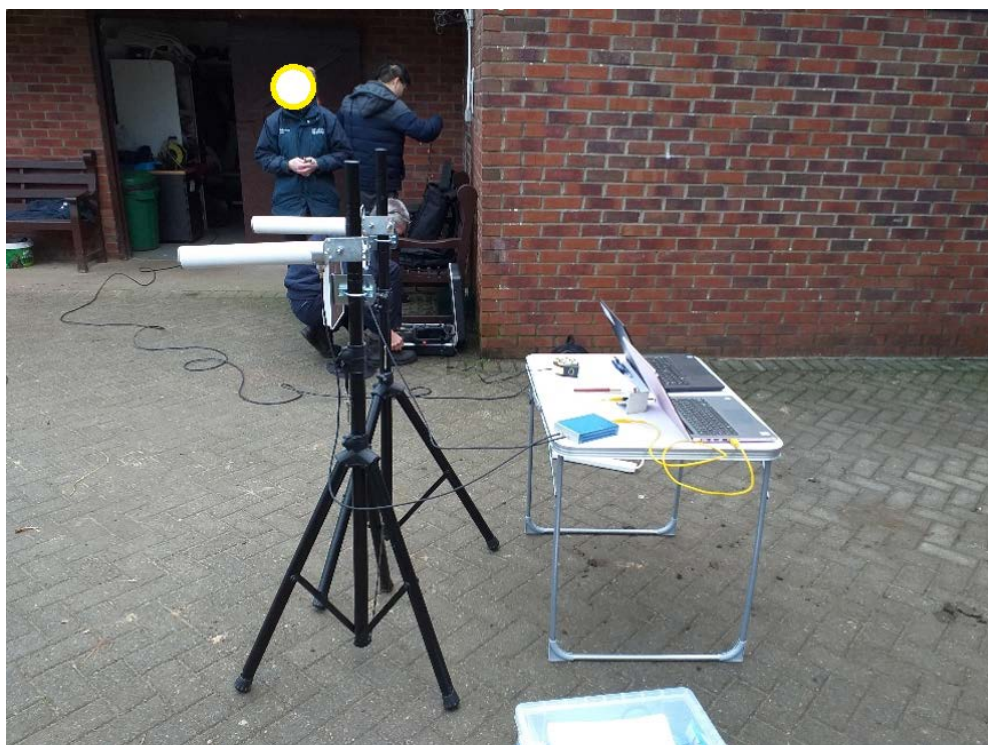
Figure 36: Radar equipment (Frequency Modulated Continuous Wave Radar) operated from a laptop for a straight-line test on hard surface in outside environment.
